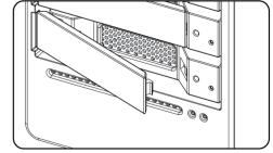
**2** Assemble the new hard disk in order and put the box back. After that, lock the box.
