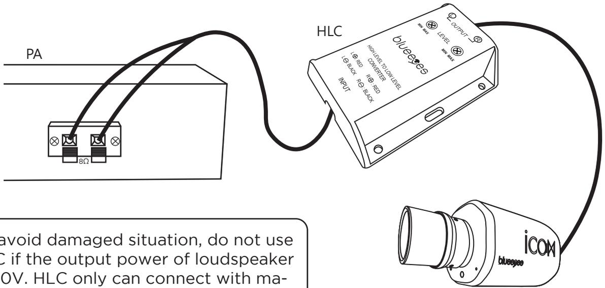
**!** To avoid damaged situation, do not use HLC if the output power of loudspeaker is 110V. HLC only can connect with machine which output is 8Ω or 16Ω. therefore, we recommend you check if there is 8Ω or 16Ω on loudspeaker or inside transformer
